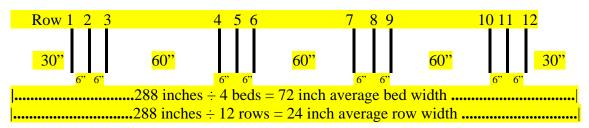
(4) From **TABLE B,** for **EXAMPLE 2** the length of the single row sample for 1/1000 acre would be 21.8 feet (24 inch average row width). The length of bed (all rows) to include in a sample would be 7.3 feet (72 inch average bed width). The combined length of sampled rows in the bed must equal the single row length. Use the sample method (single row or bed) most suitable to the field or subfield being appraised.
